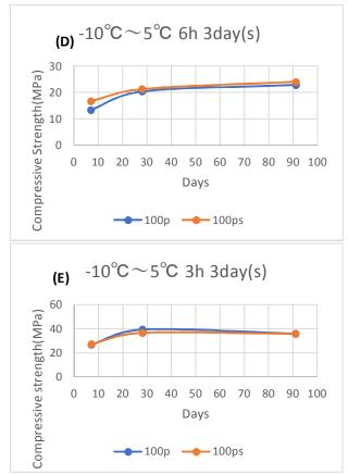
specimens was not sufficient due to the increase in the volume of water in the specimens caused by freezing and the destruction of the hardened parts by fine cracks due to the hydration reaction.
