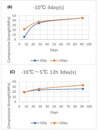
to 91 days recording an average of 45.1 MPa as shown in Fig 2B.
